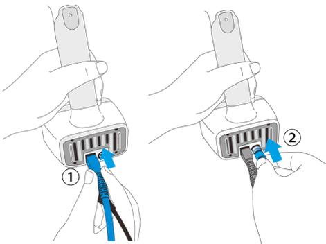
2. Plug the power cable into the connection cable.
