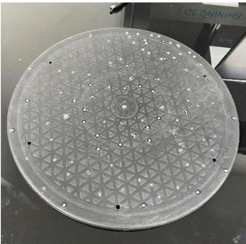
2. Put the scanned object on the center of the surface with markers, and select **Markers** alignment mode.
