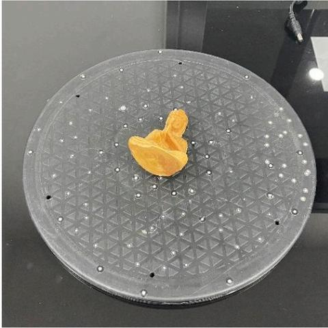
3. Turn over the object, and click **+** to create a new project within the current project group, and scan the back side of the object.
