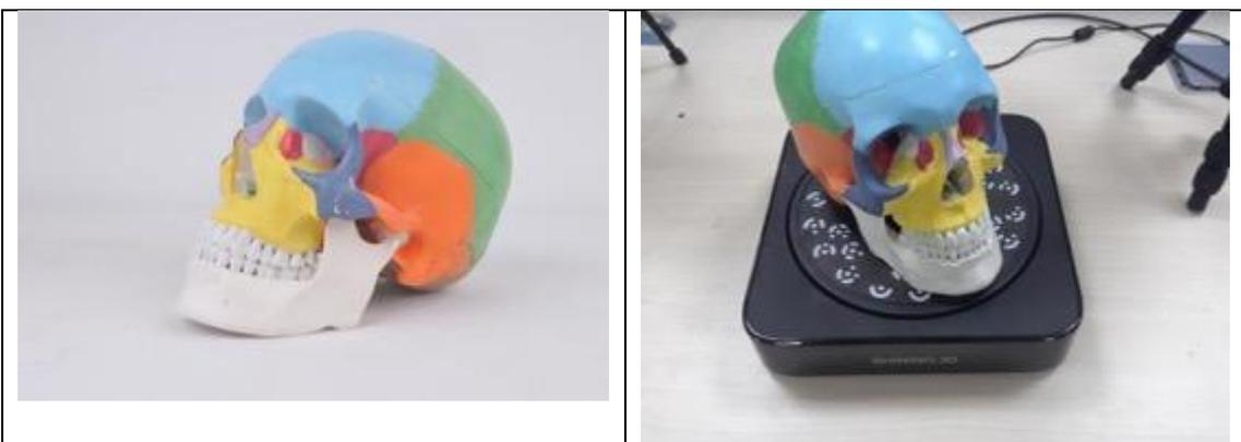
Using feature alignment, make sure that the object is kept still on the turntable, and the first view should contain enough features to allow the initialization.
