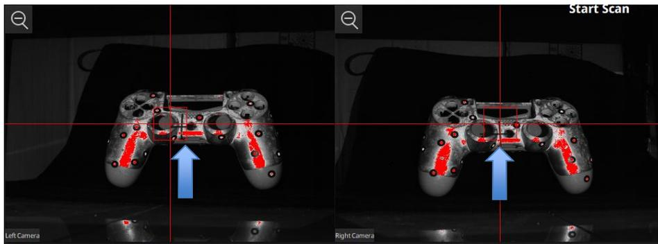
*At optimal distance the projected cross is within the central box on both cameras*
