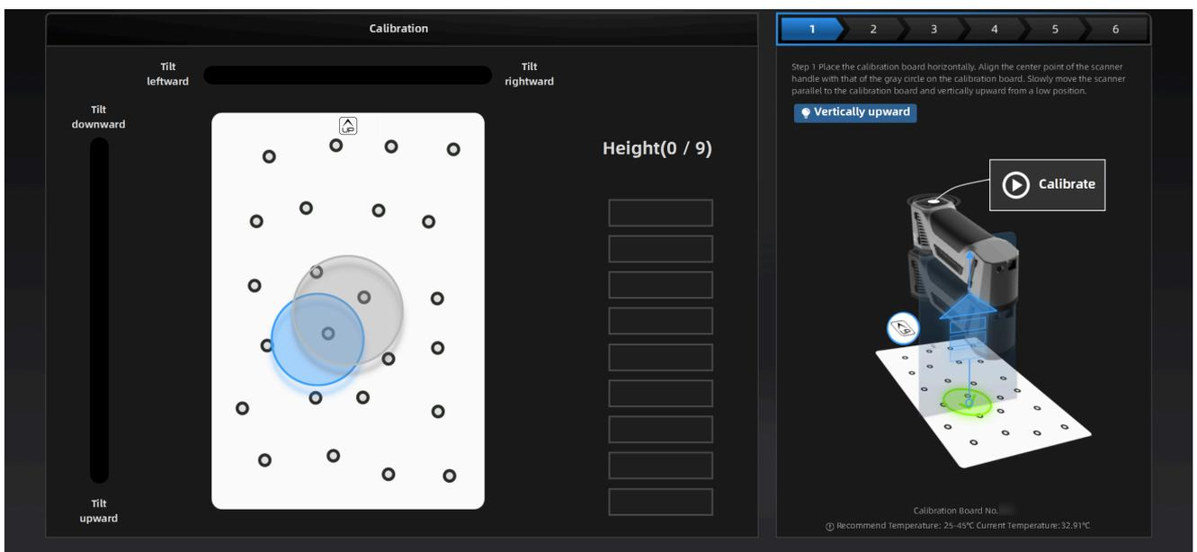
5. Move the device slowly and adjust the distance between the scanner and the calibration board according to the height indicating box.
