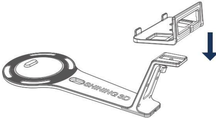
3. Mount the turntable securely onto the stand.
