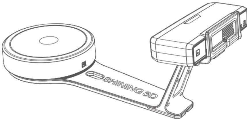
5. Connect the turnable to the scanner.
