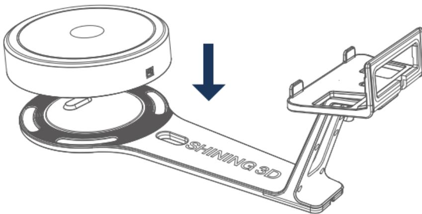
4. Attach the scanner head to the bracket.
