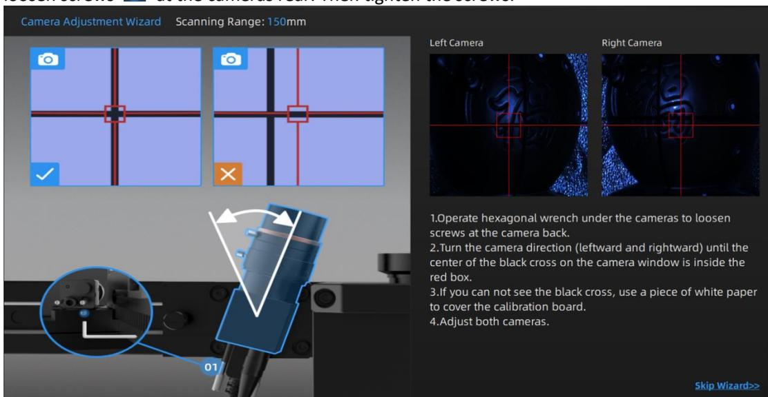
Adjust the camera aperture according to the steps shown in the following figure. Unscrew the screw on the aperture and turn the aperture to adjust the brightness of the left and right camera windows so that the white spots on the calibration board inside the viewport can be clearly seen. The recommended value is 5.6. The brightness of the camera windows is different depending on the ambient light. When the adjustment is complete, tighten the screw.
