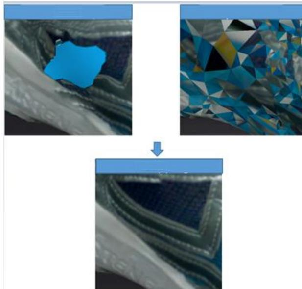
If post-processing operations have been performed, it is recommended to perform texture remapping before saving data.
