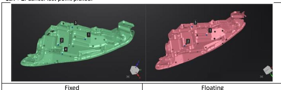
*How it works: The software calculates the best fit alignment from the picked points, and refine the alignment by best fit of all the points of the floating to the points of the fixed.*
