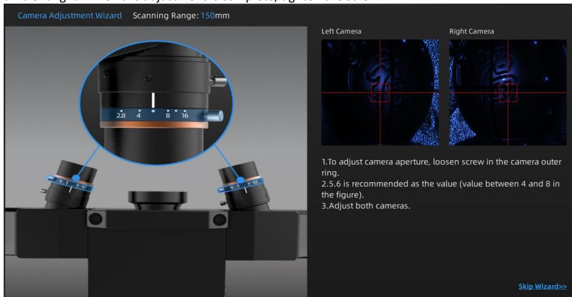
Adjust the camera clarity by following the steps in the following figure. A piece of paper with text can be placed on the calibration board to help observe clarity. Adjust to clear writing in the video stream of the left and right cameras. Double-click the left and right camera windows to zoom in and view clarity. After the adjustment is completed, tighten the screw to prevent loosening to limit the scanning effect.
