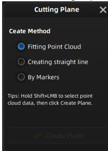
**Fitting Point cloud:** Press Shift + left-click to select data, then click the button “Generate plane”. The cut plane will be created by point cloud fitting. The direction of the plane will be calculated by the software according to the direction of point cloud.
