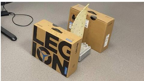
4. During the scanning process, the markers on both sides of the auxiliary objects should be scanned to complete the transition between the front and back side, then scan the lateral sides, and scan the left data after removing the auxiliary objects.
