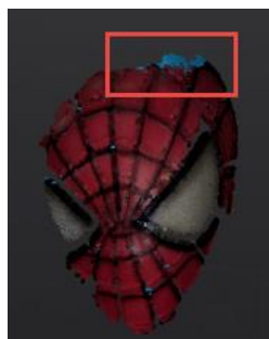
An area with texture missing
